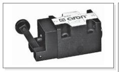
Max. pressure ports P/A/B 320 bar Max. pressure port T 160 bar 60 l/min Max. flow Minimum operating force - see note (\*) 2,5 Kg Maximum operating force - see note (\*\*) 13 Kg Cam angle 27° Fluid viscosity  $10 \div 500 \text{ mm}^2/\text{s}$ Fluid temperature -25°C ÷ 75°C Ambient temperature -25°C ÷ 60°C Max. contamination level class 10 in accordance with NAS 1638 with filter  $\beta_{25}\!\!\geq\!\!75$  •Possible mountings: E/F/G/H
