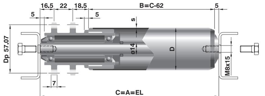
**Rulli frizionati 138 P1C - P2C con pignone in Poliammide / 138 friction rollers P1C - P2C with single or double sprocket in Polyamide**
