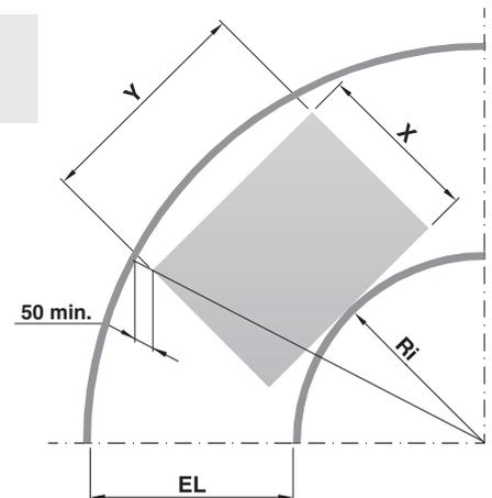
The radius of the curves with cylindrical rollers of any type is always bigger than those with tapered rollers.
